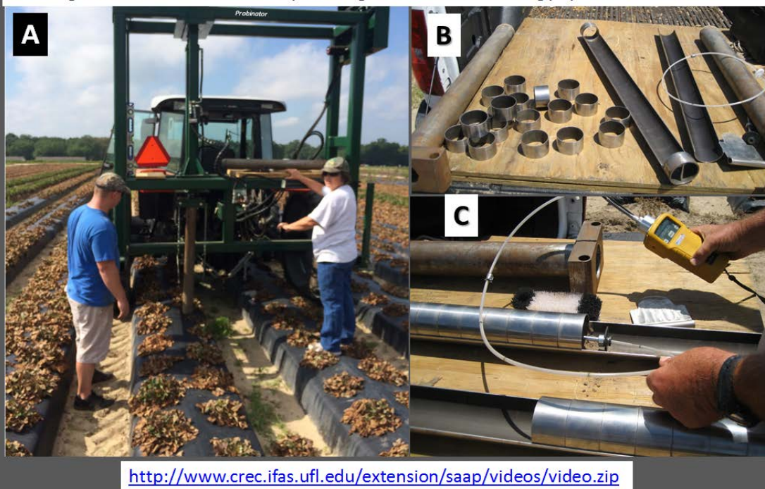
Figure 1. The Probinator (A), a hydraulically operated deep soil probe (B) used to study the depth distribution of nematodes, spatial movement of soil fumigants (C), and to identify causes of fumigant treatment inconsistency and origins of bed recolonizing populations of nematodes.
