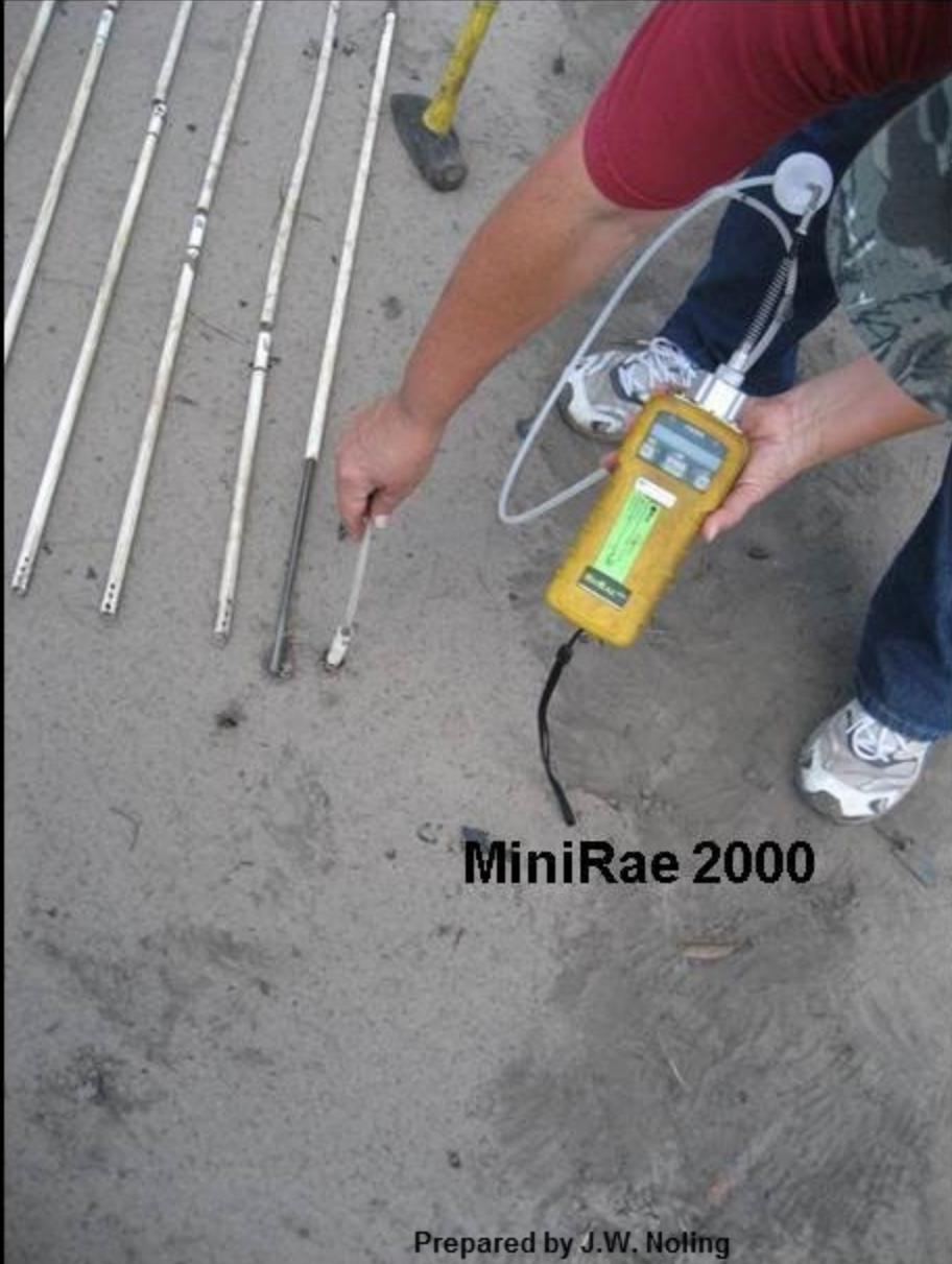
We sampled air concentrations of Telone II at multiple depths and locations using a MiniRae VOC with different soil probes
